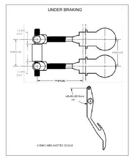
Next, find the distance between the centerlines of the front and rear master cylinders. Typically, this could be 2½ inches, but is not critical. What's critical is that this measurement, whatever it is, is exactly duplicated in the center-to-center distance of the clevises threaded onto the bias adjuster. This ensures that the master cylinder pushrods are actuated properly, minimizing any side loads applied to the master cylinder piston and bore.
