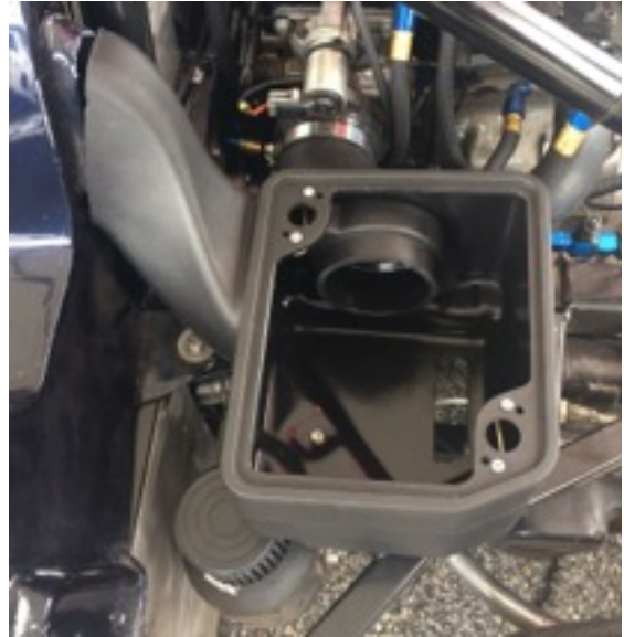
Figure 40 – Air Box Installed
