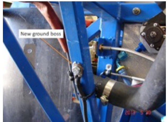
Figure 7 – Ground Boss #2 location
