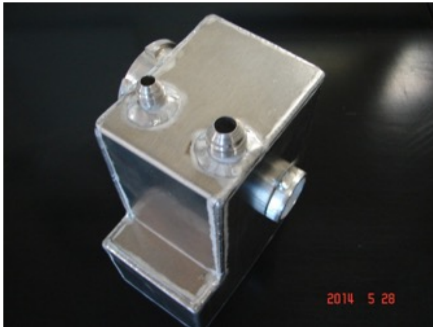
Figure 1 – Coolant Catch Tank (with new fittings and no cap)
