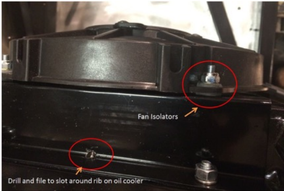
Figure 22 – Fan Mounting Bracket and Isolator
