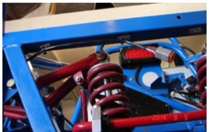
Figure 15 – Ty-wrap tabs for O2 sensor
