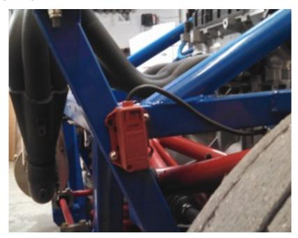
Must be securely mounted vertically as raced +/- 1.5 deg variance Must have an unobstructed view of the racing surface. Master Switch activated only
