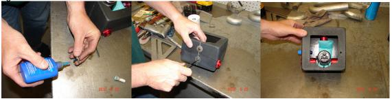
Set the box on the bench and make sure the pump is resting on the floor of the surge box and tighten the wire tie's. You can bend the filter sock and let it lay on the check valve body or place it under the check valve body directly across from the pump.
